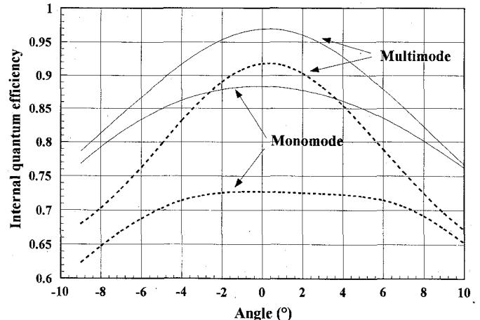
Fig. 5. Influence of the injection angle for two spot widths: continuous line: 1.3  $\mu\text{m}$ , dashed line: 2  $\mu\text{m}$ . The injection plan is ( $X, Z$ ) and when the angle increases, the light is injected toward the substrate.
