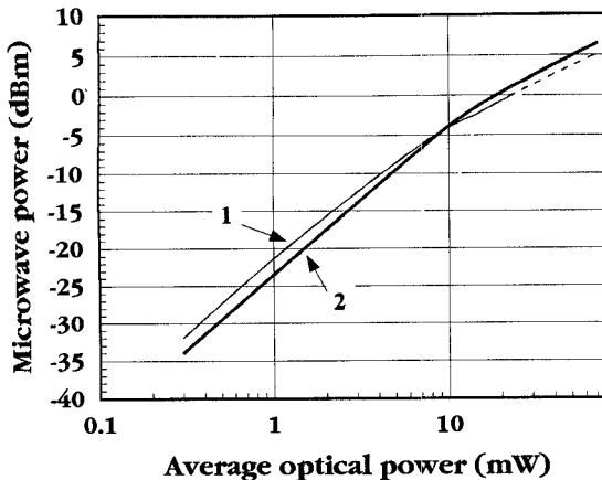
Fig. 10. Microwave responses at 60 GHz of the structure 2 ( $V_{bias} = -1$  V): 1) spot width = 2  $\mu\text{m}$ , 2) spot width = 4  $\mu\text{m}$ . The breakdown conditions are shown with dashed lines.
