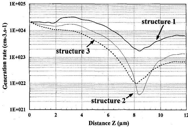
Fig. 6. Distribution of the generation rate in the structures 1, 2 and 3. The spot width is  $2 \mu\text{m}$  and the input optical power is  $1 \mu\text{W}$ .
