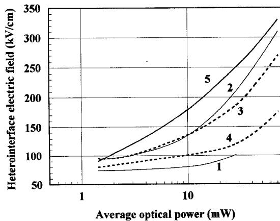
Fig. 11. Maximum electric field at the P+/N- heterointerface versus average optical power. 1) structure 1:  $V_{bias} = 0$  V spot width = 2  $\mu\text{m}$ , 2) structure 1:  $V_{bias} = -1$  V and  $W_s = 2$   $\mu\text{m}$ , 3) structure 2:  $V_{bias} = -1$  V and  $W_s = 2$   $\mu\text{m}$ , 4) structure 2:  $V_{bias} = -1$  V and  $W_s = 4$   $\mu\text{m}$ , 5) structure 3:  $V_{bias} = -2$  V and  $W_s = 2$   $\mu\text{m}$ .
