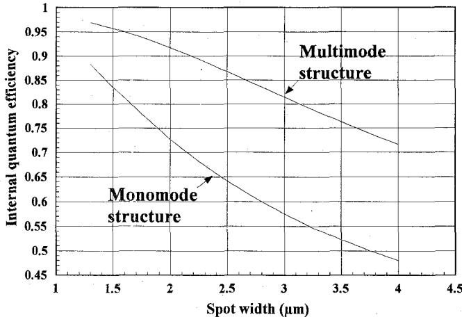
Fig. 3. Influence of the spot width on the quantum efficiency of the monomode and the multimode structure of Fig. 2.
