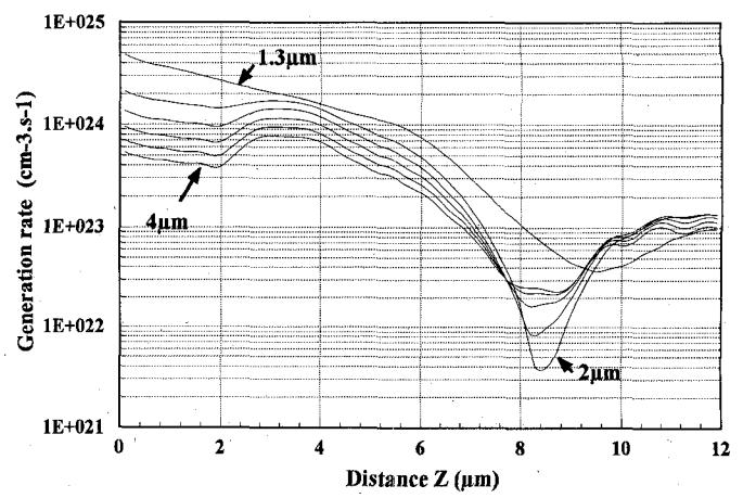
Fig. 7. Distribution of the generation rate in the structure 2 with the influence of the spot width. The spot width is successively  $1.3, 2, 2.5, 3, 3.5$  and  $4 \mu\text{m}$  and the input optical power is  $1 \mu\text{W}$ .
