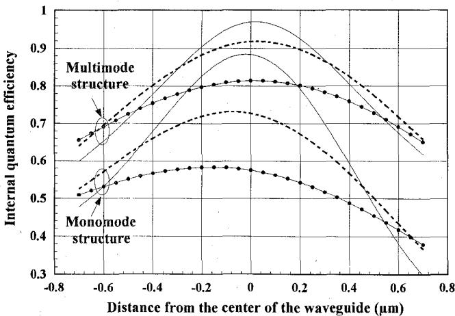
Fig. 4. Influence of the spot vertical position for different spot widths: continuous: 1.3  $\mu\text{m}$ , dashed line: 2  $\mu\text{m}$ , pointed line: 3  $\mu\text{m}$ . When  $X$  increases the light is progressively injected into the substrate.
