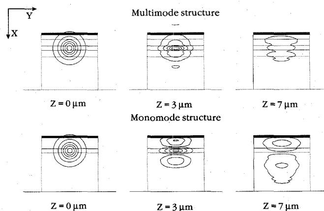
Fig. 2. Distribution of the optical energy during propagation for a monomode and a multimode waveguide PIN photodiode structure. The multimode structure is given in Table I (structure 2) and the monomode one is the same but the GaInAsP has been replaced by InP. The spot width at  $e^{-1}$  is  $2\ \mu\text{m}$ .
