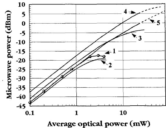
Fig. 9. Microwave responses at 60 GHz. 1) experimental results of Wake *et al.*, 2) Our results. 3) structure 1:  $V_{\text{bias}} = 0$  V and  $W_s = 2 \mu\text{m}$ , 4) structure 1:  $V_{\text{bias}} = -1$  V and  $W_s = 2 \mu\text{m}$ , 5) structure 3:  $V_{\text{bias}} = -2$  V and  $W_s = 2 \mu\text{m}$ . The breakdown conditions are shown with dashed lines.
