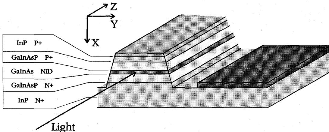
Fig. 1. Example of structure of waveguide PIN photodetector grown on InP substrate. The GaInAsP is transparent at the wavelength of injected light.
